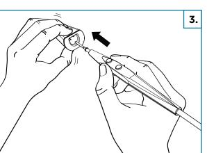
To remove the Light Jacket<sup>®</sup> from electrosurgical pencil, squeeze button with thumb until fully depressed. Remove electrosurgical pencil. Light will deactivate.
